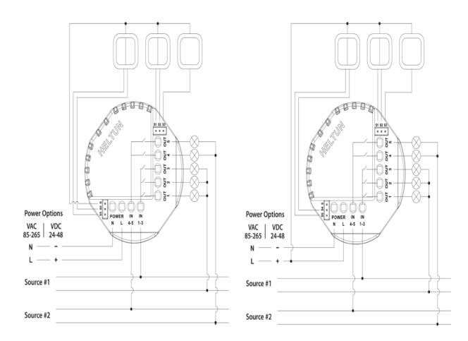
Figure 2: Power, Loads & External Switches Connection Diagram
