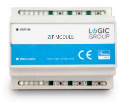
ZIF5028 is a 6 channel Z-Wave controlled DIN mountable module. The module is equipped with 6 relay switches and 6 digital inputs for mounting on a standard M36 DIN rail (EN50022).
