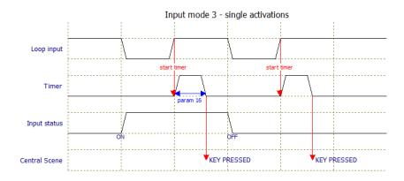
Other activation scenarios are as described in Input Mode 1, except the input status will change for each activation of the input instead of following *Loop input*.
