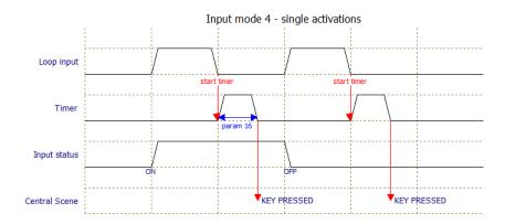
Other activations are corresponding to Input Mode 3, except the Loop Input is inverted.
