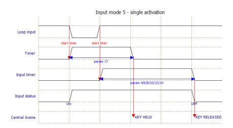
As seen from the above, a KEY HELD Central Scene notification will appear even though the activation on the input is shorter than configuration parameter 17. This is because the status on the input is prolonged with the time specified in the configuration parameter for the input timer (parameter 4/6/8/10/12/14).
