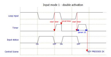
The figure above shows how a double activation is detected. The two activations must happen within the time specified in configuration parameter 16 to be accepted as a double activation.
