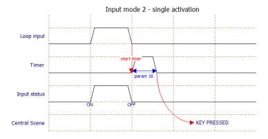
Other activations are corresponding to Input Mode 1 except *Loop Input* is inverted.
