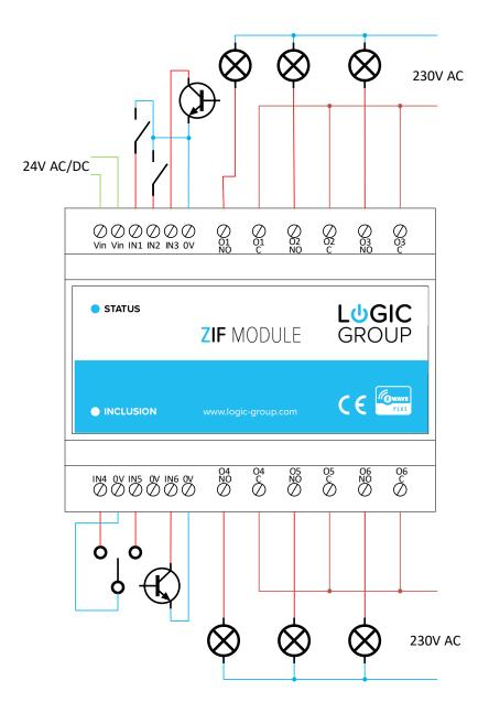
The ZIF5028 must be connected to a 24 Volt AC or DC power supply via the terminals labeled "Vin". The polarity is of no importance. The supply must be dimensioned to allow the supplied module with enough power to enable all relays to be activated. Regarding power consumption: see the technical details section.
